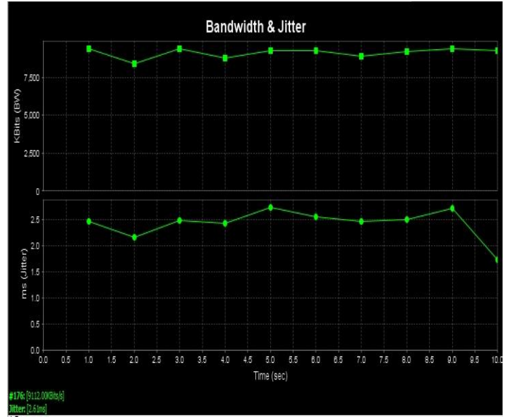
Fig. 2 UDP Test 1 with 150 mbps server and WPA2 AES.
